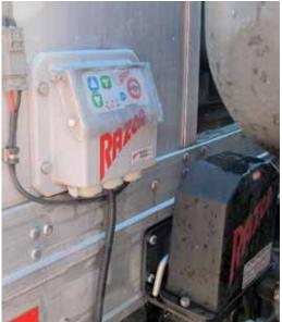
The Razor Top Runner power tarp easily operates via the switch behind the cab, or a wireless remote, and takes less than 60 seconds.
