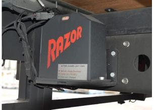
The main battery and charger is mounted out of harm's way under the chassis.
