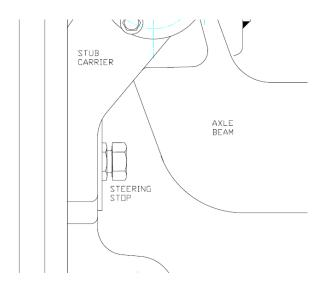
For dual tyred axles the steering stop is located in the centre of the stub carrier as shown above.
