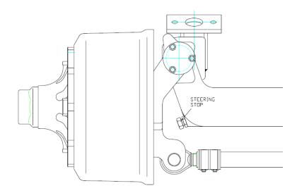
The position of the steering stop for a wide track axle is shown in the schematic above.
