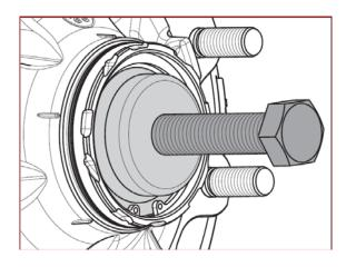
Insert the puller into the wheel hub and fit the circlip.
