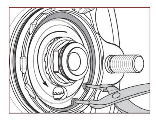
Remove the circlip from the wheel hub.
