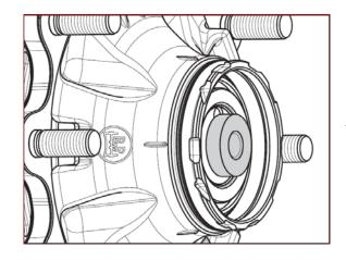
Insert the compression piece (plug) into the threaded bore.
