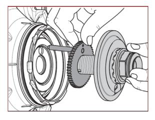
Remove the axle bolt and toothed washer with integrated pin.
