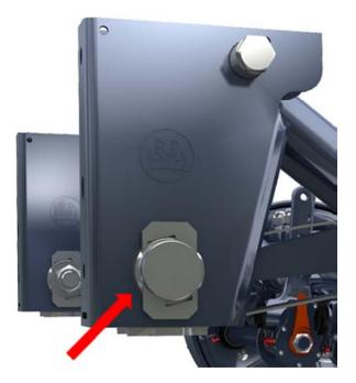
If the plates are able to be moved by hand then the bolt must be removed and the plates inspected for wear. They will normally require replacement.
