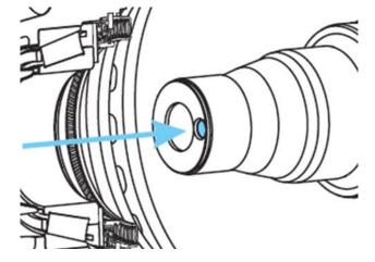
The bearing surfaces on the axle journal must be clean then have A&P (Assembly and Protection) spray applied. Ensure it is dry before assembling the hub.
