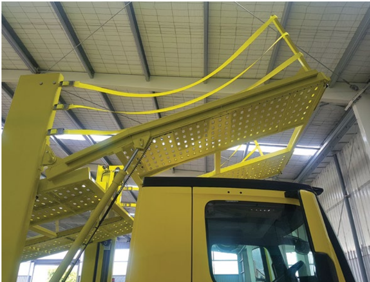
Front deck flips up to allow access to the cab for engine maintenance and servicing.
