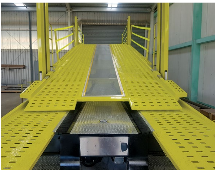
Safety mesh ensures there are minimal to no gaps to fall between when crossing the bridges.
