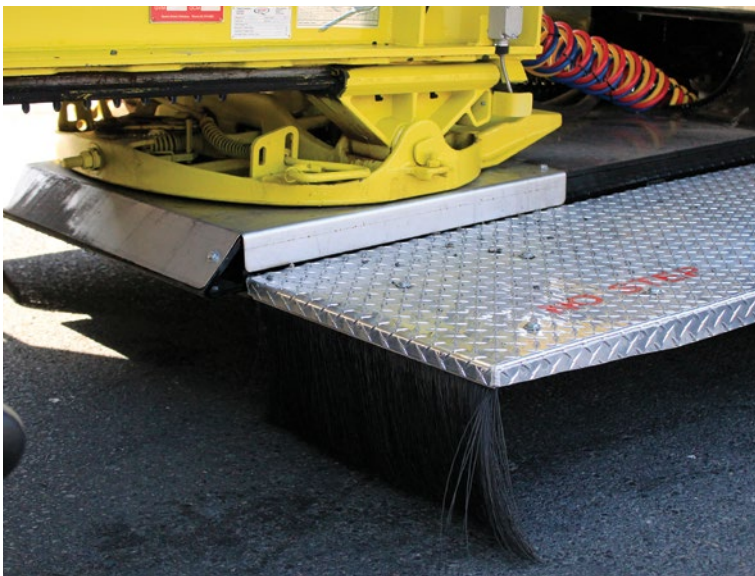
Hydraulic mid-deck is fitted with horsehair to minimise as much stone damage as possible.
