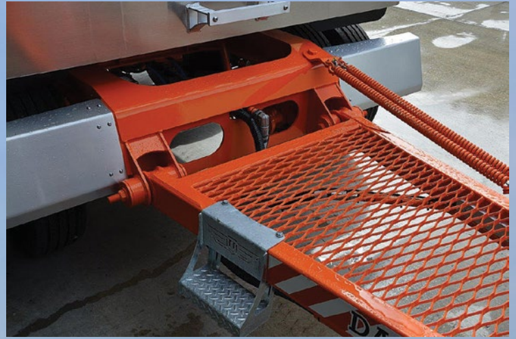
Safety mesh fitted to Drawbars to prevent fall through and removable step for ease of access
