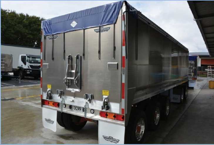
Rear door is a special feature of the Sandfords unit, with Transport Trailers working closely to build a forward-hinged, positive closing full tail door.
