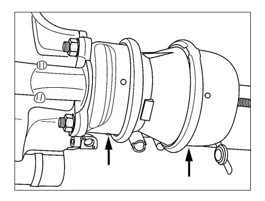
Removal of the lower bungs is important for the correct low pressure operation of the disc brake and for allowing condensate (water) to drain out. Leave all the other bungs in place.
