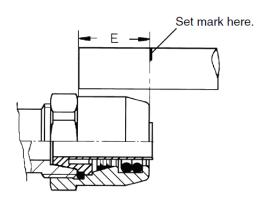
Insert the pipe into the fitting until it comes to a stop. The mark on the pipe should be parallel with the end of the fitting. Pull on the tube (20-50N) to ensure it is locked in
