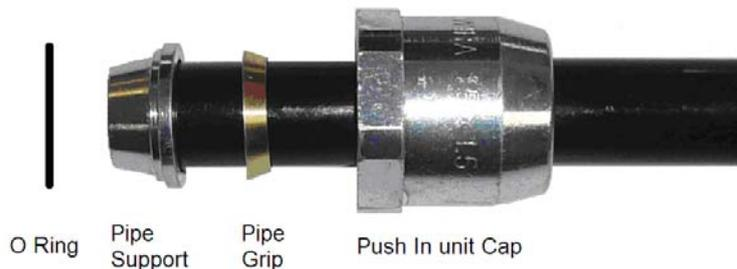
After inspecting the parts drop the pipe grip into the Push in Unit Cap with the taper facing the back of the Cap.
