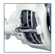
Covers can be installed during routine servicing or inspection of the disc brakes.
